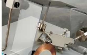
Prevents lubricant from splashing out of saw
