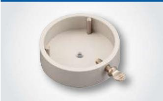
Holds mounted samples 1.5in [40mm]
